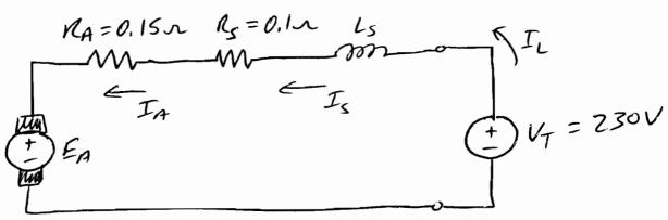
With a load drawing 20A- $E_{A_{20}} = 230 - 20(0.1 + 0.15) = 223V = K'\phi_{20} N_m$   $G = 223 = \left(\frac{0.28}{\phi_{80}}\right)(0.4\phi_{80})N_m \implies N_{m,20} = 1991.07 RPM$
