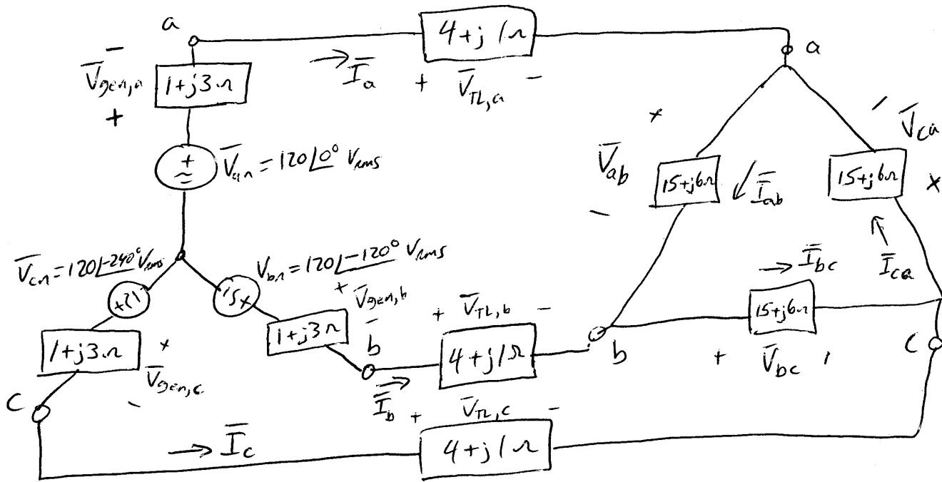
Step 1 - convert  $\Delta$ -load to  $\gamma$ -load
