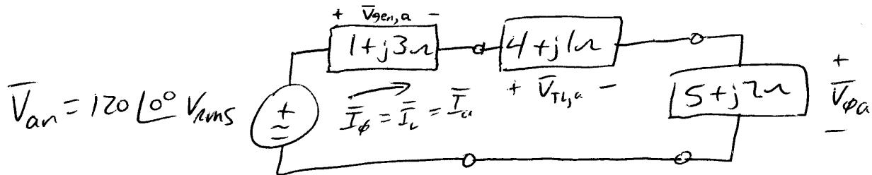
$$\bar{I}_a = \frac{120\angle 0^\circ}{(1+j3)+(4+j1)+(5+j2)} = \frac{120\angle 0^\circ}{11.6619\angle 30.9638^\circ} \text{ A}$$
