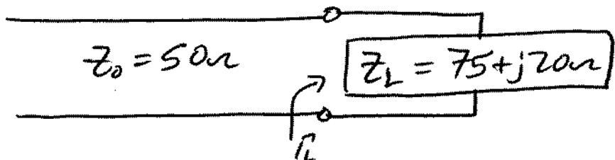
Assume coaxial cable is lossless (SWR or VSWR doesn't make much sense for lossy trans. lines)
