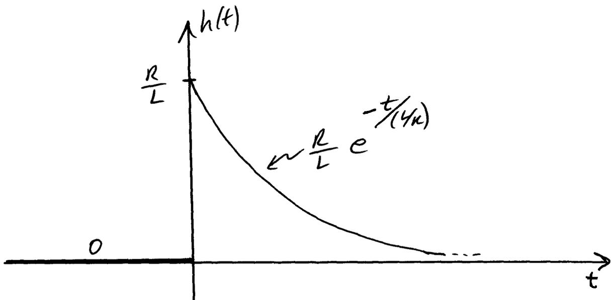
Find the output of the series RL circuit to the input  $x(t) = 5p_2(t-2)$  V when  $R=1\Omega$  and  $L=1$  H.
