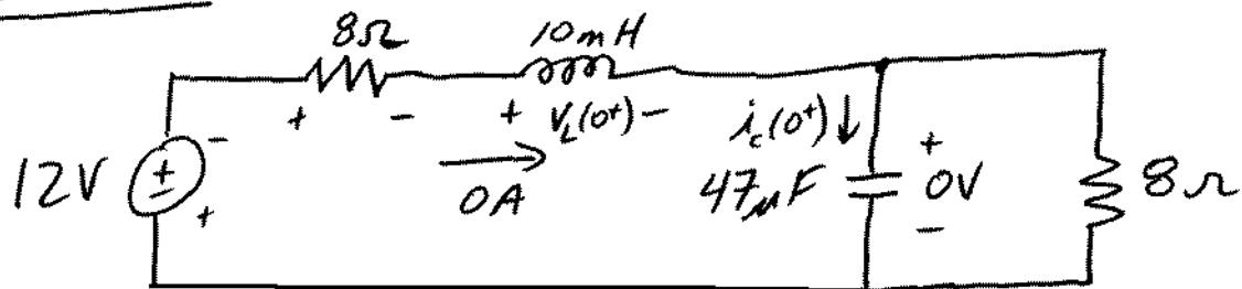
$$\text{Apply KVL} \quad -12 + 0(8\Omega) + V_L(0^+) + 0 = 0$$
