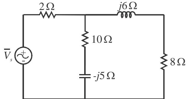
$$pf = \underline{\underline{0.9956 \text{ lagging}}} \quad P_{\text{ave}} = \underline{\underline{31.119 \text{ W}}} \quad Q = \underline{\underline{2.936 \text{ VAR}}}$$
