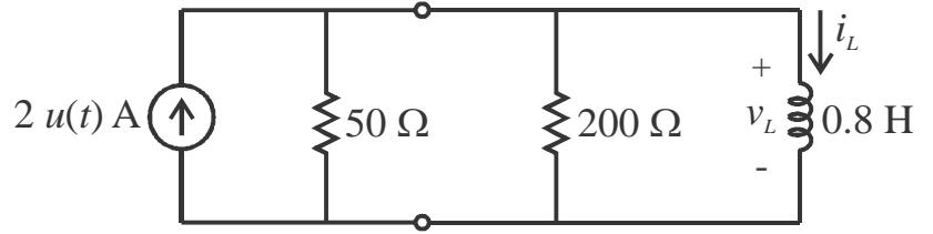
$$i_L(t) = \underline{\underline{2 - 2 e^{-50t} \text{ A } t > 0}} \quad v_L(t) = \underline{\underline{80 e^{-50t} \text{ V } t > 0}}$$
