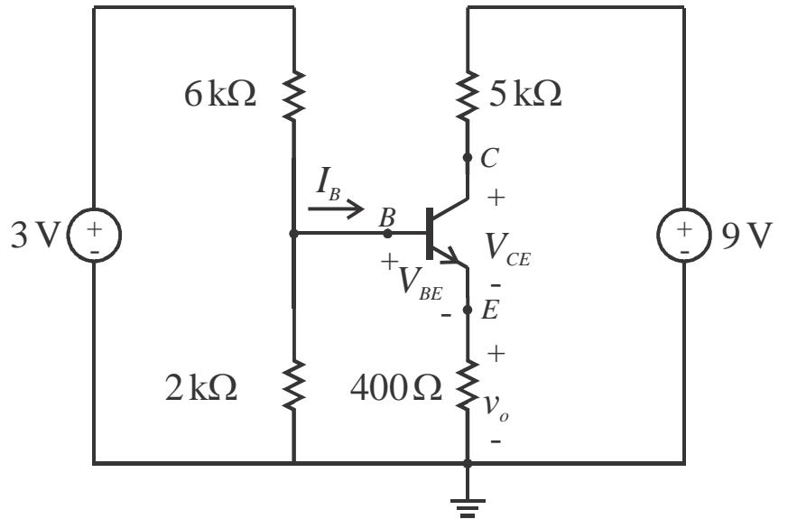
$$I_B = \underline{\underline{610.5 \text{ nA}}} \quad V_{CE} = \underline{\underline{8.34 \text{ V}}} \quad v_o = \underline{\underline{49.08 \text{ mV}}}$$
