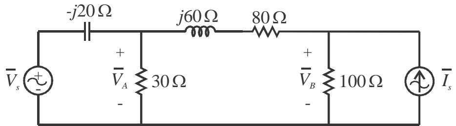
$$\underline{\bar{V}_A = 2.835\angle -20.65^\circ \text{ V}} \quad \underline{\bar{V}_B = 27.18\angle 15.78^\circ \text{ V}}$$
