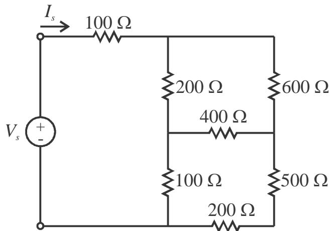
$$R_{\text{eq}} = \underline{\underline{340.625 \Omega}} \quad I_S = \underline{\underline{70.46 \text{ mA}}}$$
