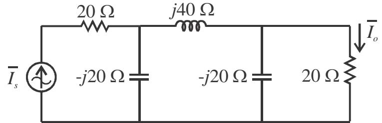
$$\bar{Z}_{eq} = \underline{\underline{40 - j 40 \Omega}} \quad \bar{I}_o = \underline{\underline{500 \angle 180^\circ \text{ mA}}} \underline{\underline{}}$$
