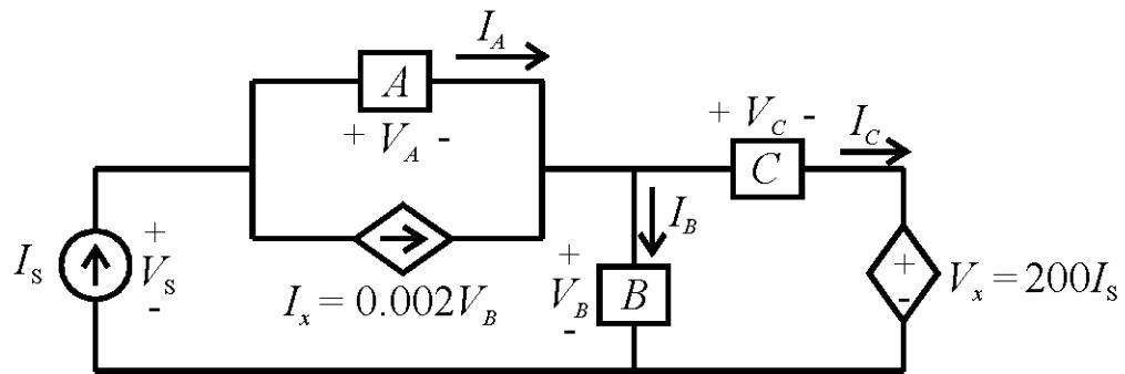
$$V_C = \underline{13 \text{ V}} \quad V_S = \underline{25 \text{ V}} \quad V_x = \underline{5 \text{ V}} \quad P_A = \underline{-77 \text{ mW}}$$
