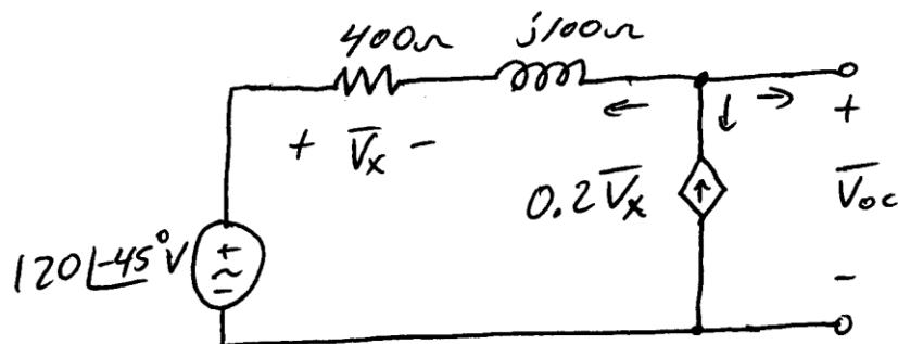
$$\text{Apply KCL to top right node : } \frac{\bar{V}_{oc} - 120\angle -45^\circ}{400 + j100} - 0.2\bar{V}_x + 0 = 0$$
