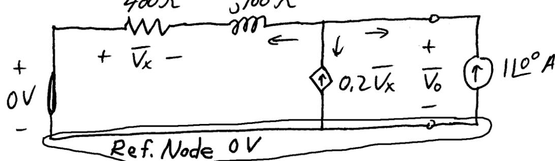
$$\text{Apply KCL to top right node: } \frac{\bar{V}_o - 0}{400 + j100} - 0.2\bar{V}_x - 1L^{\circ} = 0$$
